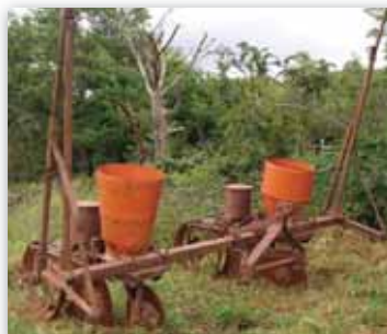
An example of an old planter converted to do no-till planting.
